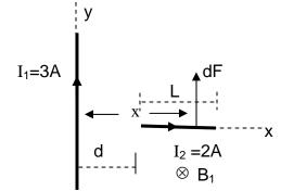
$$dF = I_2 dx \ B_1 = I_2 \frac{\mu_o I_1}{2\pi x} dx$$
