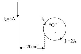
$$B_1 = \frac{\mu_o I_1}{2R} = 6.28 \times 10^{-6} T \otimes, B_2 = \frac{\mu_o I_2}{2\pi r} = \frac{M_o I_2}{2\pi (0.4)} = 2.5 \times 10^{-6} T \odot$$
