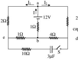
2 $\Omega$ For the circuit shown the switch S is open and the capacitor is uncharged. Find: (a)- The current I. d Left loop 1:  $12 = I + 3I_1$ Right loop 2:  $12 = I + 6I_2$   $I_1 = 2I_2$   $12 = (I_1 + I_2) + 3I_1$ ,  $I_2 = \frac{12}{9}A$ ,  $I_1 = \frac{24}{9}A$  $\therefore I = 4A$
