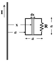
[6 Marks] b) Show that the magnetic flux through the square loop is given as:  $\Phi = \frac{\mu_0 I a}{2\pi} \ln(2)$
