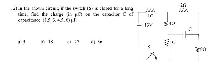
13) In the previous circuit of question 12, if the switch S is now opened at t = 0, find the time (in  $\mu$ s) required for the capacitor to lost (25%, 35%, 45%, 55%) of its initial charge.
